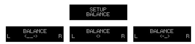
Left channel is increased with regards to right channel by rotating the encoder counter clockwise or by pushing the "arrow left" key on the remote control; right channel is increased with regards to left channel by rotating the encoder clockwise or pushing the "arrow right" key on the remote control.
